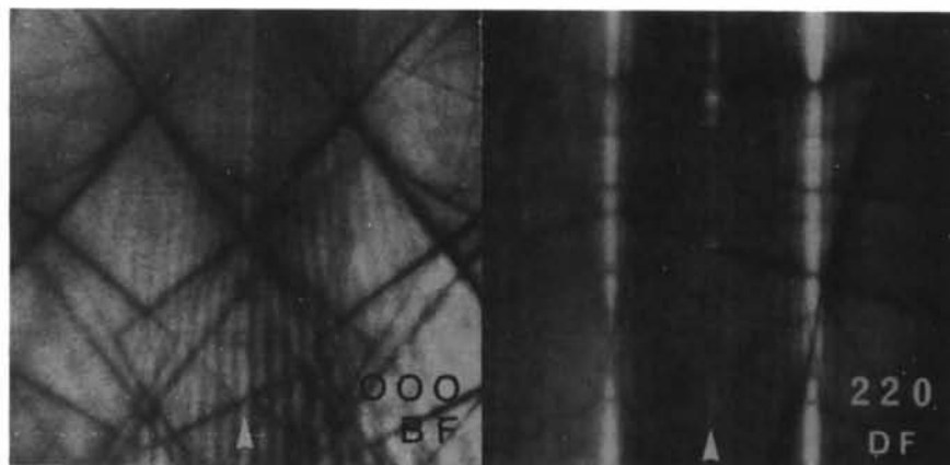
Fig. 1. Diffraction conditions for critical voltages: ( a ) 110 systematic critical voltage; ( b ) nonsystematic critical voltage at the 150 reflection in the [513] zone; ( c ) [113]-zone-axis critical voltage; ( d ) nonsystematic critical voltage at 002 in the [100] zone.
